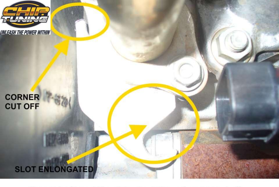
For easier fitment the plate should have 1 corner cut off it and the opposite side filed down slightly so it slides past the bolts.
