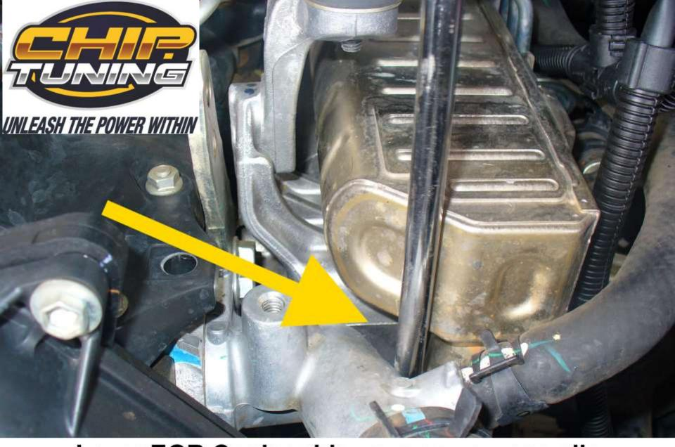
Lever EGR Cooler sideways so you can slip in the EGR Blanking Plate
