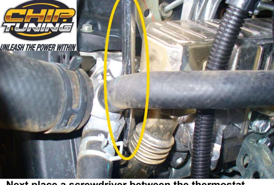
Next place a screwdriver between the thermostat housing & EGR Cooler pipe & lever it sideways.(Cont)
