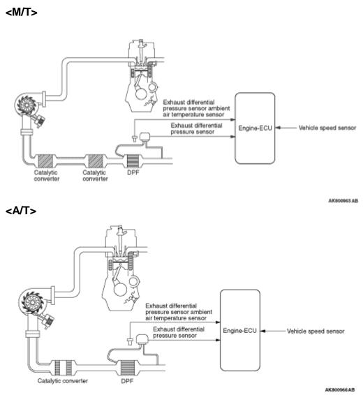
Calculating the input signal sent from each sensor, the engine-ECU anticipates the amount of PM accumulated in the DPF. The anticipation method is as follows:
