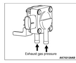
The exhaust differential pressure sensor is installed around the upper area of the DPF. Using the piezo resistive semiconductor, the exhaust differential pressure sensor outputs the voltage to the engine-ECU in accordance with the difference in the voltage between the DPF upstream area and the DPF downstream area. The engine-ECU anticipates the amount of PM accumulated in the DPF through this output voltage. The sensor characteristics are as shown in the charts.
