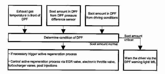
The ECM receives information about the soot amount accumulated in the diesel particulate filter from the DPF pressure difference sensor. In addition, the ECM calculates the soot amount in the filter from the driving conditions of the vehicle.
