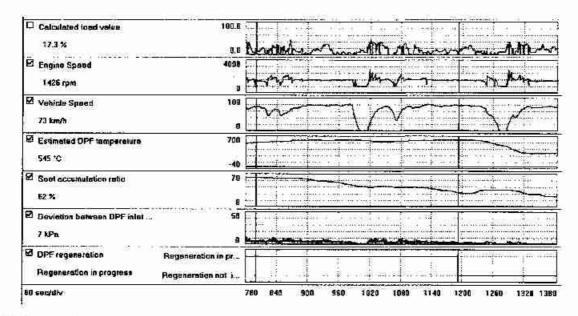
NOTE: During the active regeneration process the drivability, engine revolutions, engine sound and exhaust gas smell may change. In addition, it is possible for white smoke to be emitted from the exhaust tailpipe during regeneration. These are side effects of the regeneration process and should not be considered as a concern.
